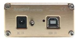
USB input Connect to host PC with a suitable 2.0 USB cable with a Female B USB connector.
