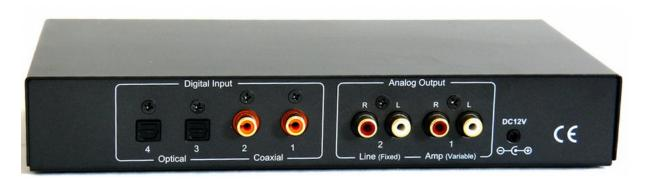
If directly connecting the TC-7510 to amplified speakers or power amps, use the "Variable" mode.
