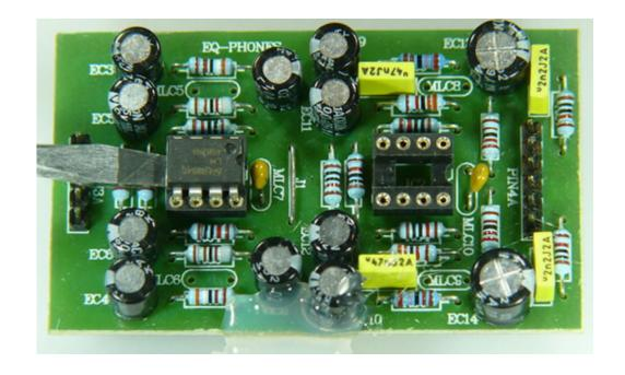
Now put the opamp into the socket on the Gator PCB. Please make sure that you place it in the same position as in the picture. **DO NOT FIT IT IN THE WRONG WAY ROUND!** The writing on the opamp should be upside down when seen from the front of the DAC.
