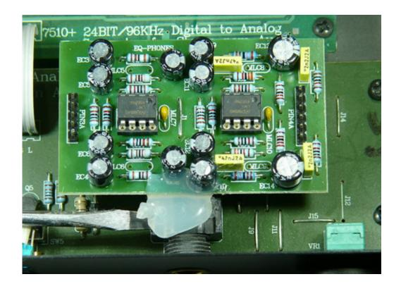
Lift the PCB upwards. You might need toi use some extra force since the PCB is secured to the headphone socket via double sided tape, as well as the glue.
