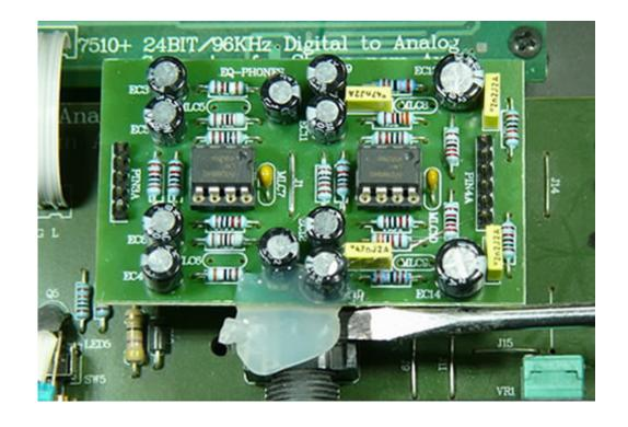
Use the screwdriver to separate the glue on the right side as well.
